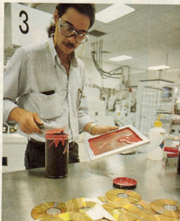
(ABOVE) At the JVC Disc America Company in Tuscaloosa, Alabama, music is made, not played, by machines such as this one. (RIGHT) JVC America employee David Cannon ensures a colorful disc label by applying shocking red paint to a silk screen. To add to the glitz, aluminum or 24-karat gold is melted and used to coat discs in a process called "sputtering."
