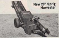
The popular new 20" Sprig Harvester digs and loads 400 to 500 bu. of clean sprigs per hr. Up to 600-900 bu. with side loading elevator. Same rugged construction as larger models. Interchangeable parts.
